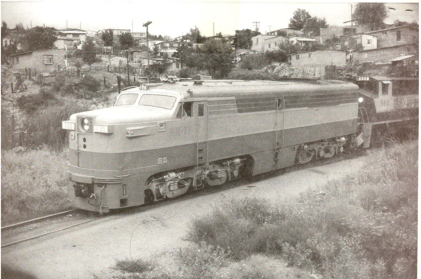
FNM DH-17 (ALCO PA-1) pulling a special train of 150 railfans on a “Let’s Travel Tours” tour east of Nogales, Sonora, Mexico on September 28, 1990. The DH-17 was thought to have been scrapped, but was actually rebuilt at Empalme (with 40-inch wheels instead of 42-inch). Meanwhile, DH-19, the other FNM PA-1, had been put in a museum in Puebla at this time. Both these engines were from the Delaware & Hudson Rwy (DH-17 was formerly Santa Fe #60L built in November 1948). The special also had engines #563 (Bombardier), #539 (GE), and RS11 #501 (former Pacifica) hauling five passenger cars and a caboose. (Photo by Peter Smykla, Jr, first published in the November 1990 Arkansas Railroader)
