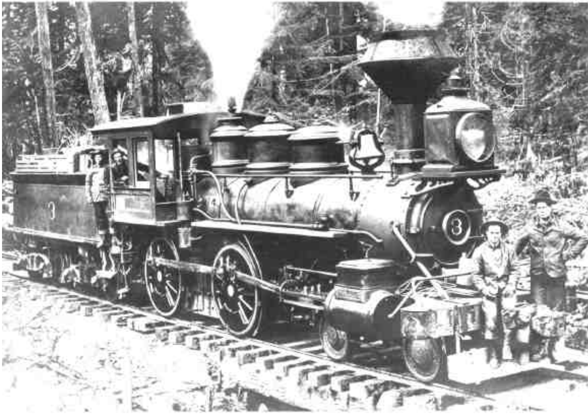
Diamond stack 4-4-0 No. 3 has a Union Pacific “brand” on her right steam chest, but she was operating on the old Oregon Railway & Navigation road, probably in 1890s.
